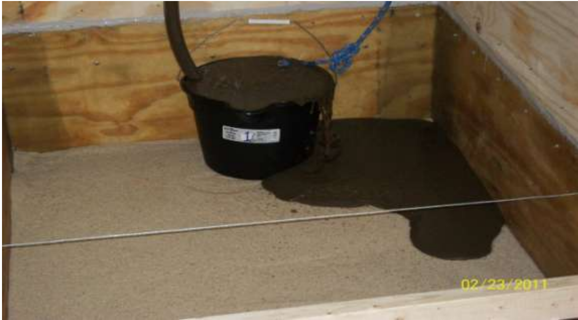
Figure 2.3 Sludge application point in pilot-scale bed
