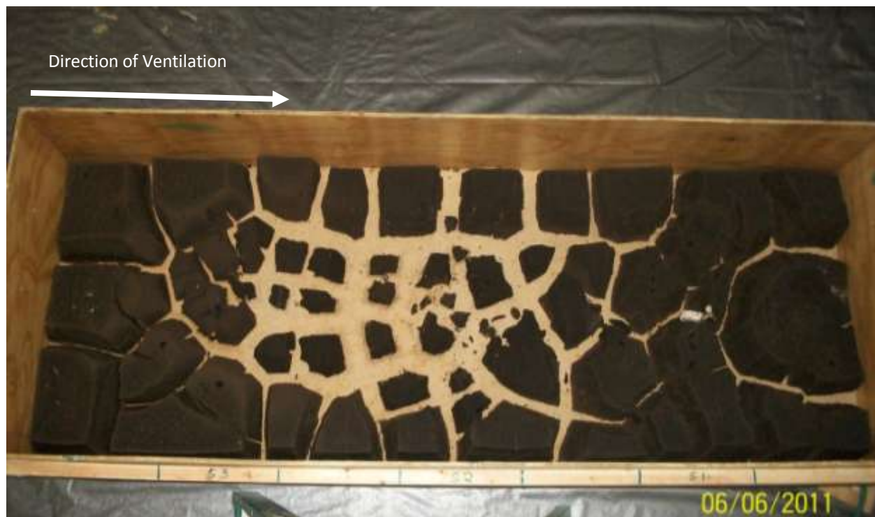
Figure 3.5 Sludge cracking observed in Bed 3 at the end of Ventilation Test 3 (1 fan @ 300 cfm)
