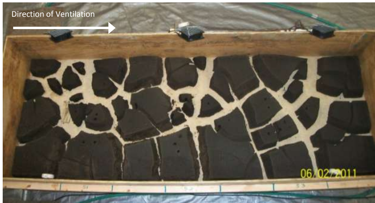
Figure 3.4 Sludge cracking observed in Bed 2 at the end of Ventilation Test 3 (3 fans @ 100 cfm each)
