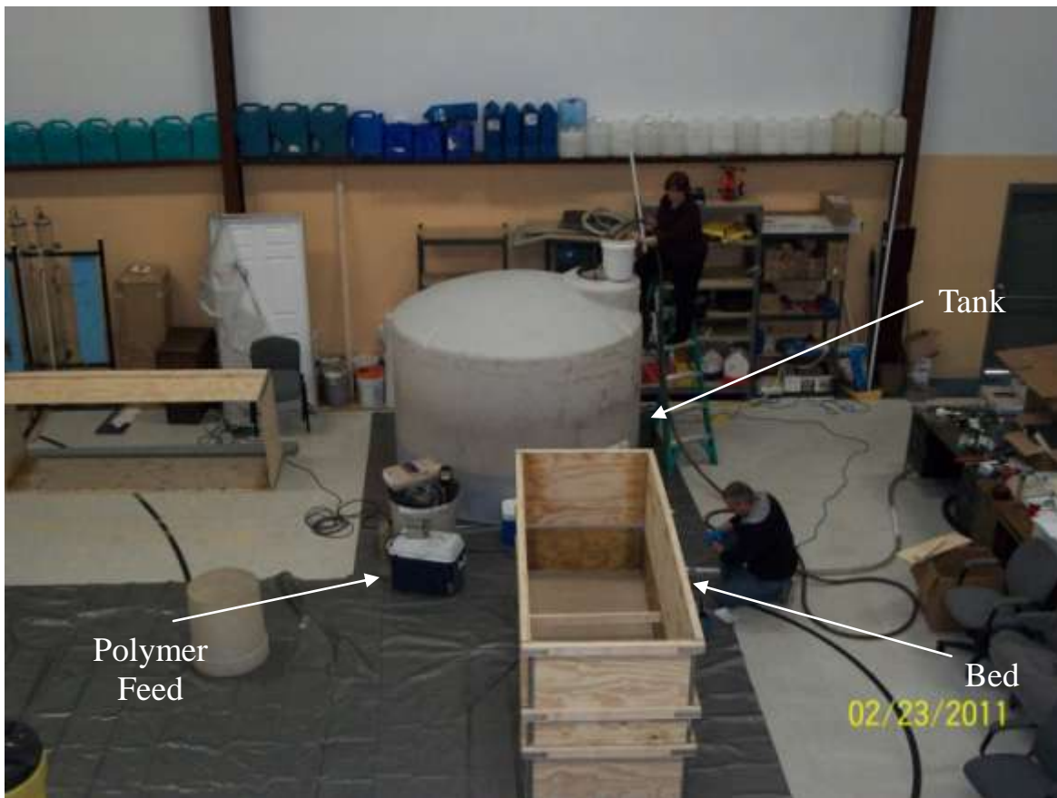
Figure 2.4 Experimental apparatus setup with one pilot-scale bed
