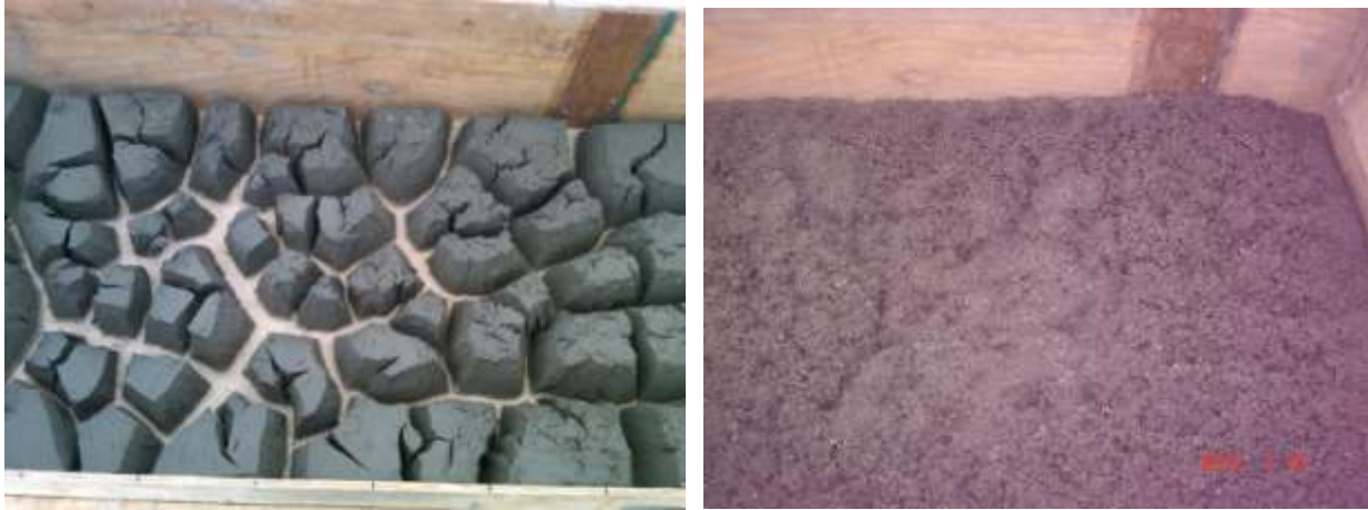
Figure 3.24 Comparison of West Bed after 13 days of dewatering during Cleveland Test 1 (left photo) to West Bed after six days of dewatering during Cleveland Test 3 (right photo)
