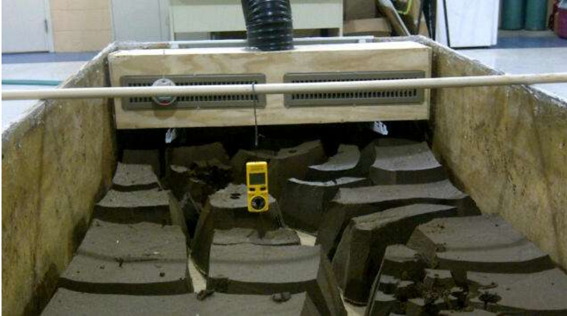
Figure 2.11 Air velocity measurement apparatus
