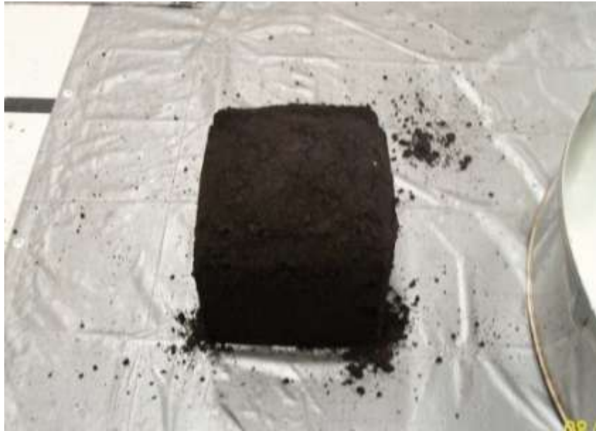
Figure 3.13 Pile 1 on Drying Day 1 (12-inch x12-inch x12-inch)
